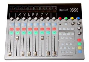
The Master Control Surface (MCS) has 8 'channel strips' (faders) and monitor and talkback controls
