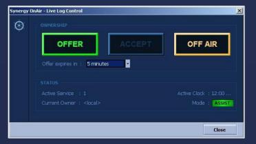
The messaging system is also used with Clydes' ARCS software — Audio Router Control System, which manages station-wide audio routing in a multi-studio multi-service environment, controlling an external router — analog or digital, with however many inputs and outputs are required.
