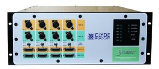
The MPU is the 'engine' which undertakes audio processing – in effect a digital audio mixer.
