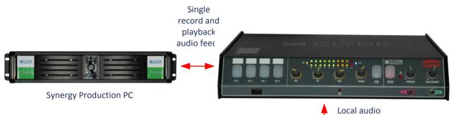
The main purpose of the Production/Back Up Workstation is for 'production' – recording, editing, production, scheduling and admin, with optional traffic tools i.e. the creation of content which will be broadcast at a later date.
